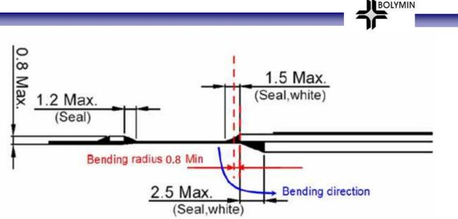
12.5 Avoid bending the film at IC bonding area.(>1.5mm)(this could damage the ILB bonding)
